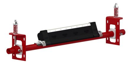
The MUS2 secondary cleaner is unique within itself to have a parallelogram designed into the cushion allowing constant blade angle attacking to the material flow, this allows for automatic adjustability within the cleaner for when the belt thickness can vary. The MUS2 is well suited for conveyor belts with mechanical fasteners when the (TI) tungsten impact blade is applied. For Vulcanised belt MATO recommend the (TL) tungsten long-life blade
